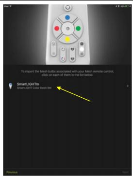
13. In this screen, the lamps associated with the remote control are listed. You must configure each of these bulbs one by one using the installation wizard.
