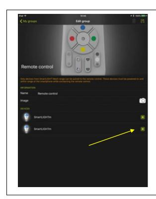
2. Uncheck the bulb that you want to disassociate from the remote control.
